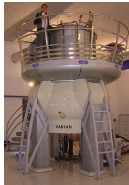
A 900MHz NMR instrument with a 21.2 T magnet at HWB-NMR, Bir-
